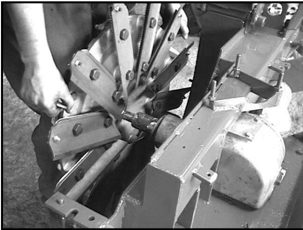
Picture 16. Pulling apart the flywheel
