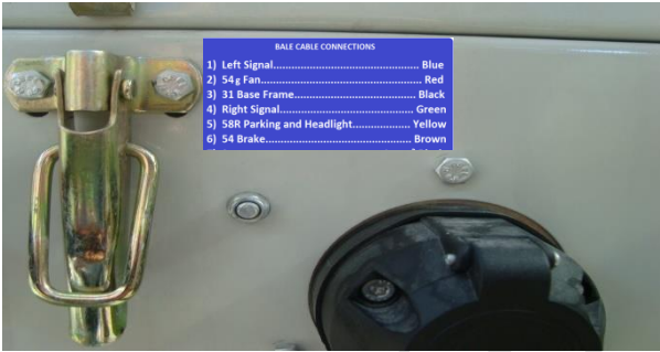
Figure 16: Power connection outlet
