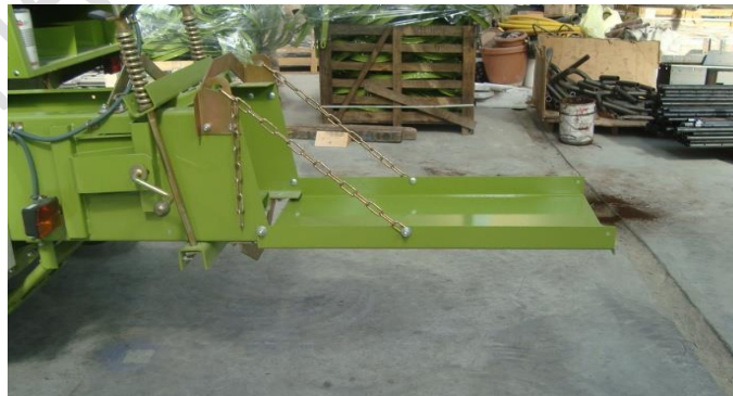
Figure 23: Bale Outlet Hatch
