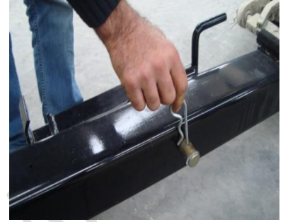
Figure 7: Jack safety pin
