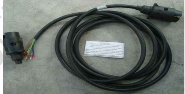
Figure 17: Electric connection cable
