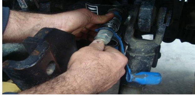
Figure 15: Connection of Hydraulic Hoses to Tractor
