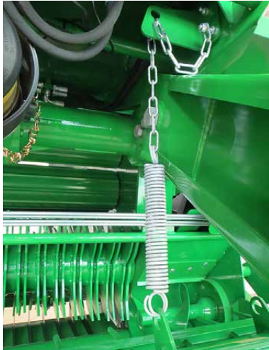
Crop guard adjustment chain & plate
