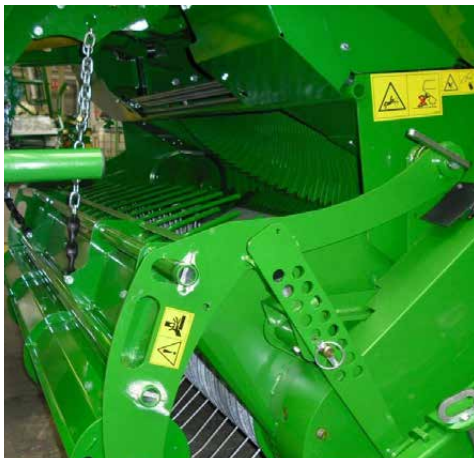
Crop roller adjustment chain
