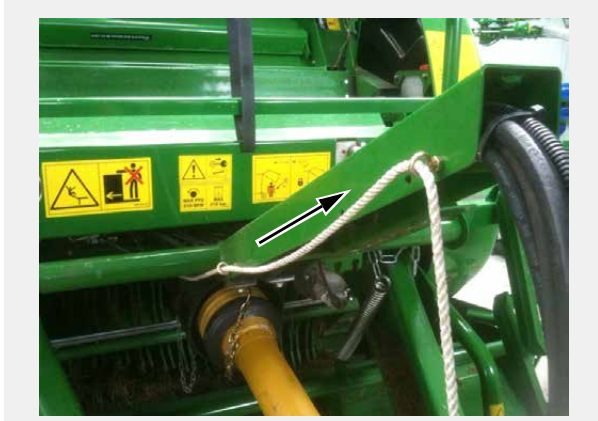
To activate the drop floor, pull the cord towards the tractor, whilst operating the pick-up spool-valve lever
