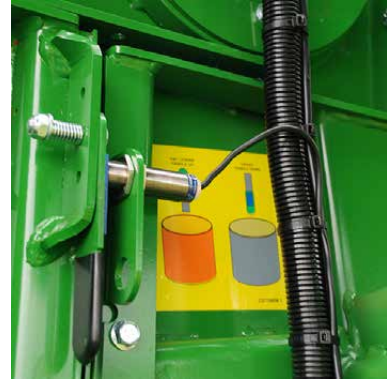
Grass & silage position (handle down)
