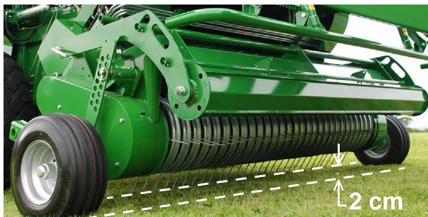
Pick-up reel height adjustment
