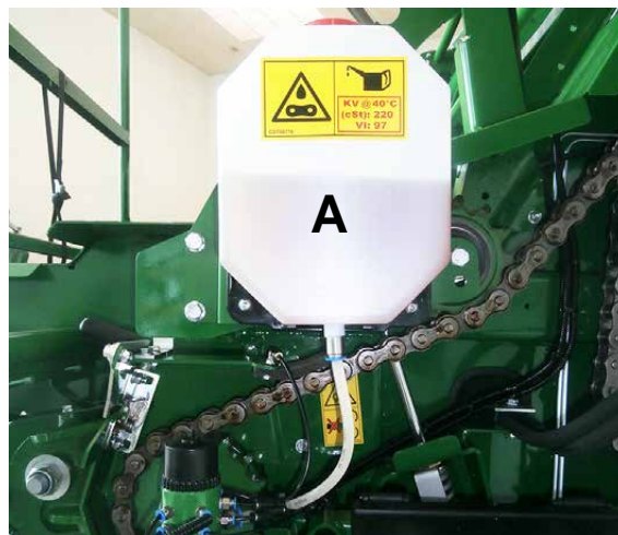
Oil reservoir tank
