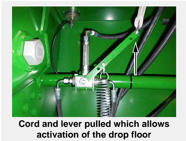
To activate the drop floor, pull the cord towards the tractor, whilst operating the pick-up spool-valve lever
