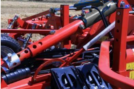
Hydraulic parallel lifting
