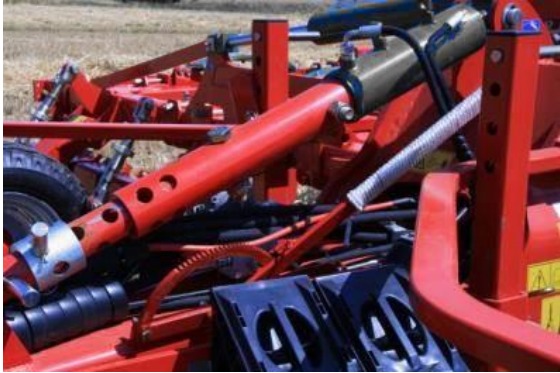
Hydraulic parallel lifting
