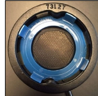
Figure 17: Ultrasonic Sensor with Mesh
