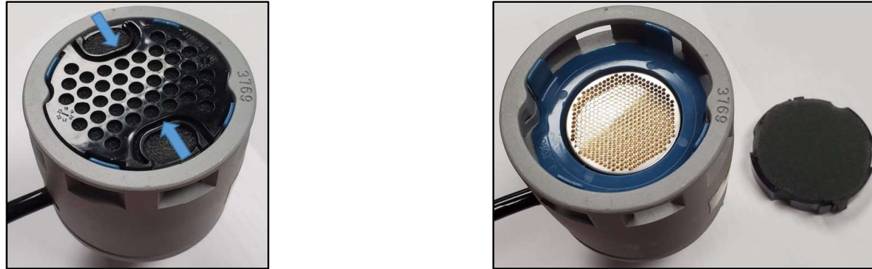
Figure 18: Sensor Foam Retainer Clip Removal
