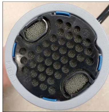
Figure 16: Ultrasonic Sensor with Retainer Clip
