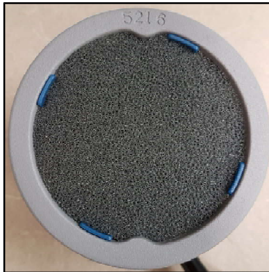
Figure 15: Ultrasonic Sensor with Foam
